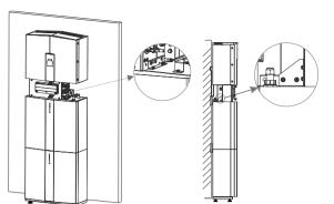
Figure 11 Inverter Installation on the Wall
