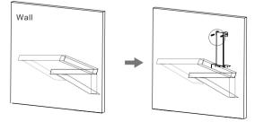
Figure 13 assemble the inverter mounting panel on the tripod angle support
