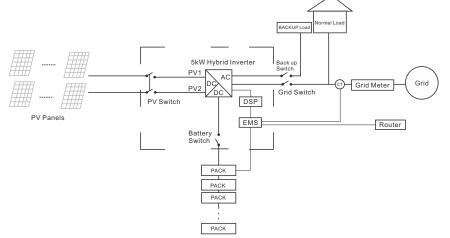
BACKUP L 5kW Hybrid Inverter Back up Switch AC Grid Meter Grid Grid Switch DSP EMS Router Battery Switch \ PV Meter PACK PACK PV Inverter **PV** Panels PACK PACK
