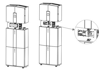
Step 1: Turn on the external PV switch.
