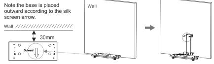
Figure 9 Base installation diagram
