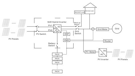
Figure 29 Hybrid-coupled system
