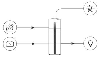
• **BAT PRIORITY:** Under this mode, the battery is only used as a backup power supply when the grid fails and as long as the grid works, the batteries won't be used to power the loads. The battery will get charged with the power generated by the PV system or from the grid.
