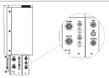
Figure 17 Cable Box Bottom View, Wiring Connectors Step 9 Note: this step only suitable when use HEC-S B 5/10/15/20K batter pack. Take out the communication cable set provided in the accessory parts of one H5/H3-BAT, cut o ffone end and crimp a new RJ45 connector. If there are two batteries, you only need to remake one of battery communication cable on site.
