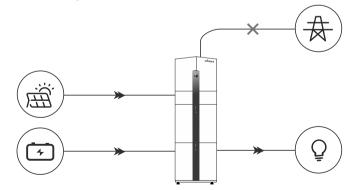
• **PEAK SHIFT:** This mode is designed for time-use mode customer. The customer is able to set up the charging/discharging time & power via inverter screen or APP.
