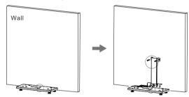
Figure 12 assemble the inverter mounting panel on the base Step 6 Hang the inverter onto the inverter mounting panel as Step 4
