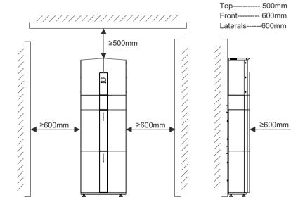
Figure 8 Limited Distance of Installation to Neighboring Objects
